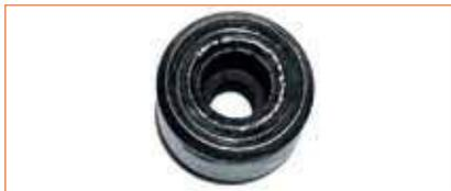
interior ring damaged for 100%
